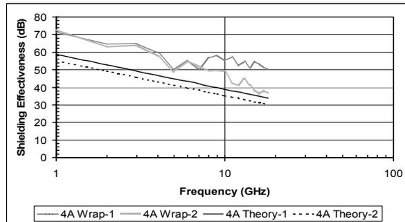
Figure 5. Measured and Calculated Stirred Mode Shielding Effectiveness of Sample 4a.
