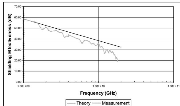
Figure 8. Measured and Calculated Stirred Mode Shielding Effectiveness of Type N Barrel with Two Apertures
