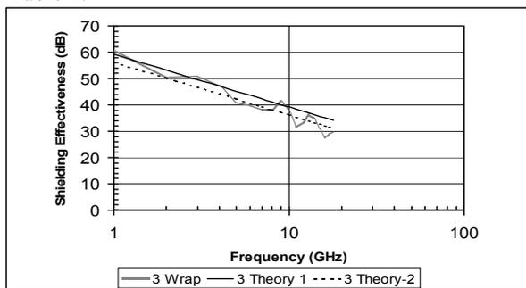
Figure 2. Measured and Calculated Stirred Mode Shielding Effectiveness of Sample 3.
