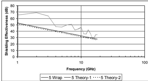
Figure 6. Measured and Calculated Stirred Mode Shielding Effectiveness of Sample 5.
