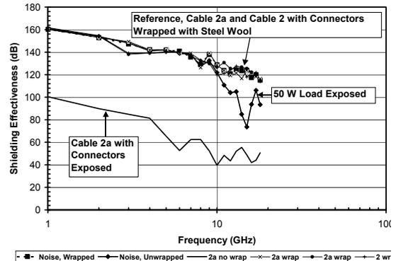
**Figure 1. Initial Stirred Mode Shielding Effectiveness Measurements of Samples without Apertures**
