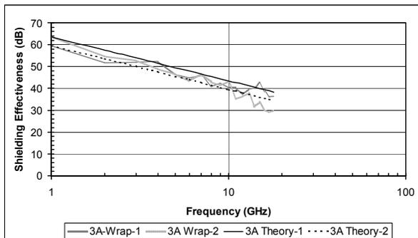
Figure 3. Measured and Calculated Stirred Mode Shielding Effectiveness of Sample 3a.
