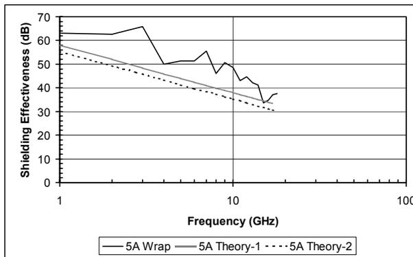
Figure 7. Measured and Calculated Stirred Mode Shielding Effectiveness of Sample 5a.
